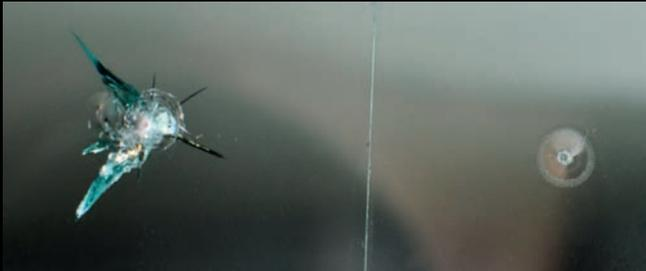
the image to the left shows the results of a rock hitting an unprotected windscreen at 60mph. On the right is the result of the same impact on a windscreen protected by ClearPlex invisible windscreen protection film. The impact leaves only a small dimple in the film, but does not nick or chip the windscreen glass underneath, leaving it in pristine condition.
